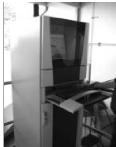
Computer Terminals – This terminal control soil sorting bins and overhead rail storage system.
