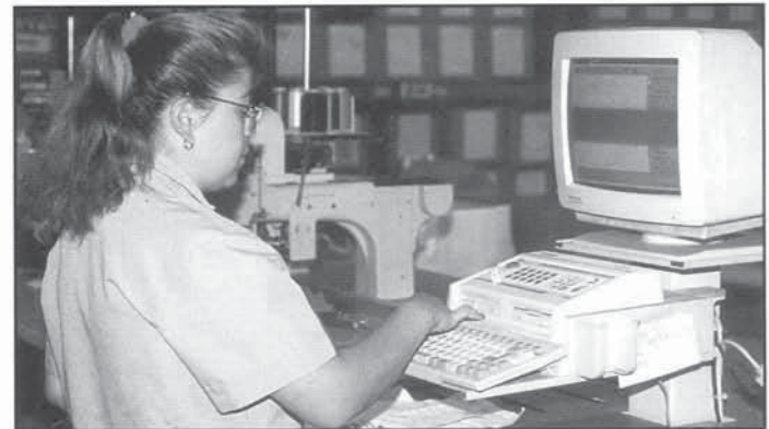
A computer is used to send instructions directly to the 6-head embroidery machine.
