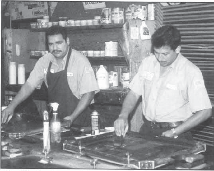
The Plant has its own silk screening equipment for badges and emblems.
