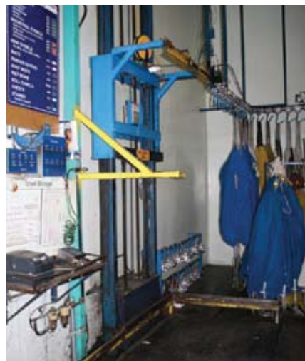
A sign on a wall in the plant advises employees on drying schedules for various goods coming from 450 and 800 lb. washers. An automatic lift raises up slings of soiled goods to the overhead rail system for movement to the wash aisle.
