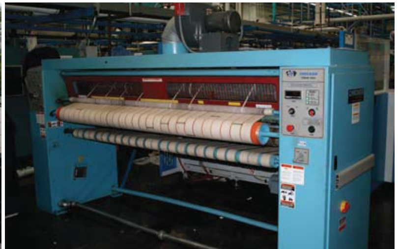
An ironer from Chicago Dryer Co. is used to process a growing number of napkins that are processed in the plant.
