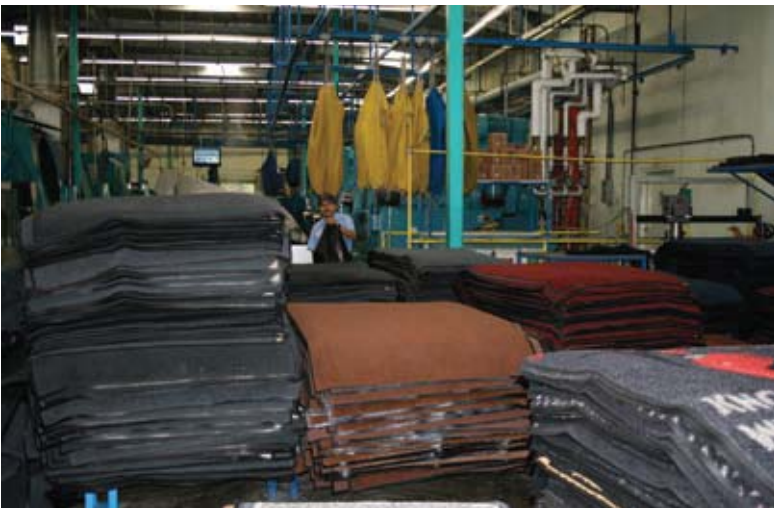
POS stores clean mats flat rather than rolling them. This makes for more efficient movement onto the trucks with less labor.
