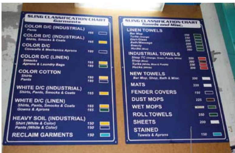
Signs posted in the plant indicate which goods go in what color of slings. The color-coding system helps everyone know instantly what types of goods are in a given sling as it moves through the plant.
