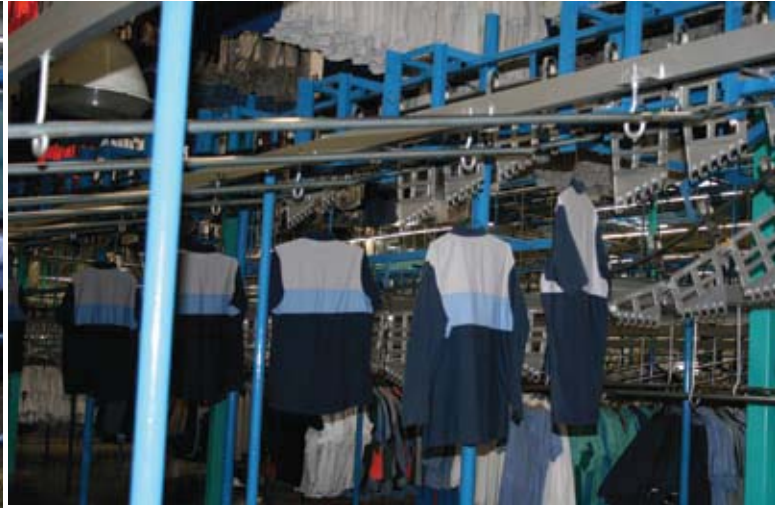
Work shirts move on an overhead rail system through the finishing department.
