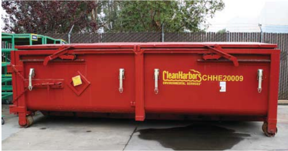
POS/Vista deposits dry sludge from its wastewater treatment system into the metal container shown above. The bin is taken to a landfill and emptied about three times a year.
