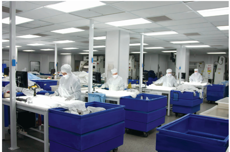
Housekeeping, as discussed in ISO 14644-5, keeps this ISO Class 8 (FED-STD-209 Class 100,000) immaculate on both a visual and microscopic level. Pictured is a PCS soil sort room.
